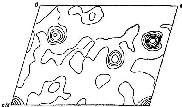
Fig. 4. Fourier projection on (010) using 86 reflexions with signs determined from inequalities and sign relationships. Contours at equal, arbitrary intervals.
